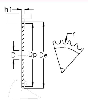
C = 4 D = 30 De = 611.7 Dp = 596.55 For chain size = 1 1/4 x 3/4 For chain type = 20 B-1 h1 = 18.5 Sumber of teeth = 59
